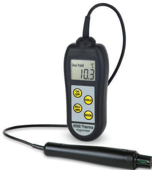
**INSTRUMENT OPERATION** - The instrument is switched on by pressing the ON/OFF button. To obtain accurate humidity measurements, allow the instrument to stabilise in the environment for a minimum of one minute. To maximise accuracy, allow airflow across the sensor.
